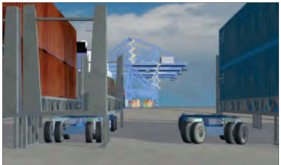
Figure 1: C-AGV turning 90 degrees in the direction of a loaded cassette
