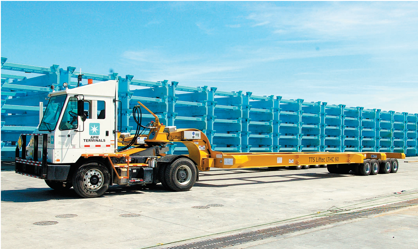
A manual version for handling containers using cassettes and AGVs has recently been implemented at APM Terminals' new US east coast hub in Portsmouth, Virginia
